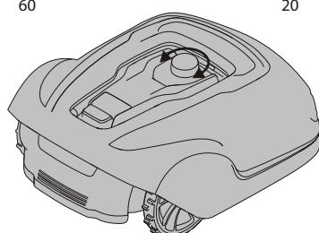
For the first few weeks of mowing, set the cutting height to 60 mm to avoid cutting the boundary wire and guide wire. Lower the setting one step each week thereafter until the desired cutting height is reached.
