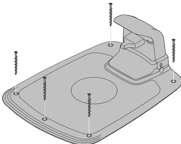
Secure the charging station to the ground using the five supplied fixing screws using a 6 mm hex key.
